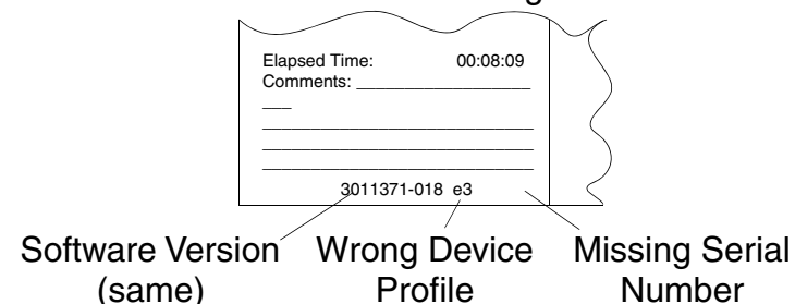
Device with incorrect configuration data
